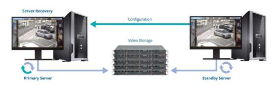
**Failover quickly switches** to a standby server when communication with the primary server is lost. The standby server automatically takes over all functions from the offline or malfunctioning server. Live video streaming and recording resume immediately. You can suspend any server in the cluster with no system downtime, e.g. for maintenance.
